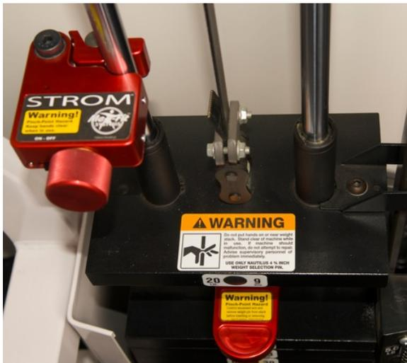
The start point module is slid into one of the adjustment holes on the top plate and stem, eliminating the additional weight of simply pinning into the stack, and providing an extra measure of safety for clinician and patient.
